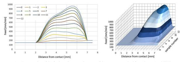
Fig. 12. Formation of the feed rate in successive tests of the recurrent method for a short Ø4.5 drill bit
