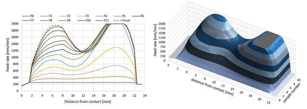
Fig. 10. Formation of the feed rate in successive tests of the recurrent method for a long Ø8 drill bit
