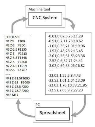
Fig. 4. Data exchange in a recursive loop
