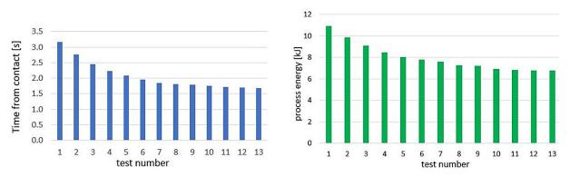
Fig. 13. Drilling process time and power consumption in successive tests for a short Ø4.5 mm drill bit
