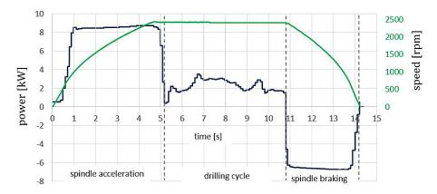
Fig. 14. Power consumption in successive phases of the friction drilling process
