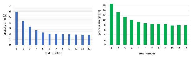
Fig. 11. Process time and energy demand in successive steps of the recursive method for a Ø8 drill bit
