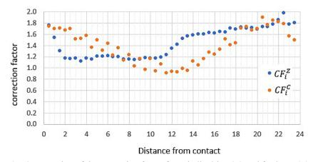
Fig. 6. Formation of the correction factor for spindle drive (C) and feed rate (Z)
