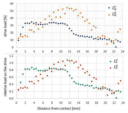
Fig. 5. Example of a spindle drive load and feed drive load distribution
