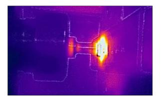
Fig 1. Friction drilling monitoring with an infrared camera
