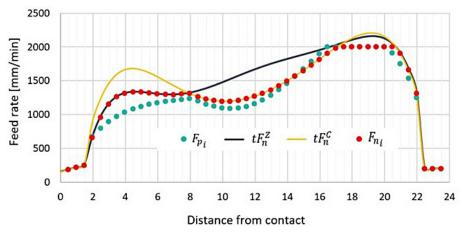
**Fig. 8.** Example of determining a feed table in the next  $F_{n}$  test
