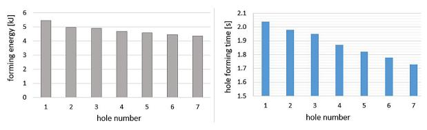
Fig. 16. Energy consumption and hole formation time for a series of 7 consecutively drilled Ø8 holes with active adaptive control
