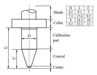
Fig. 9. Shape and basic dimensions of the drills used in the tests
