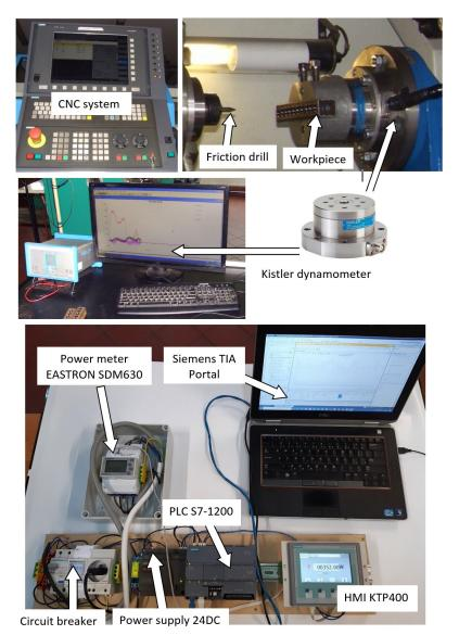
Fig. 3. Test rig for measuring energy consumption during friction drilling
