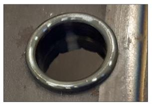
Fig 2. Collar and bushing of friction drilled hole
